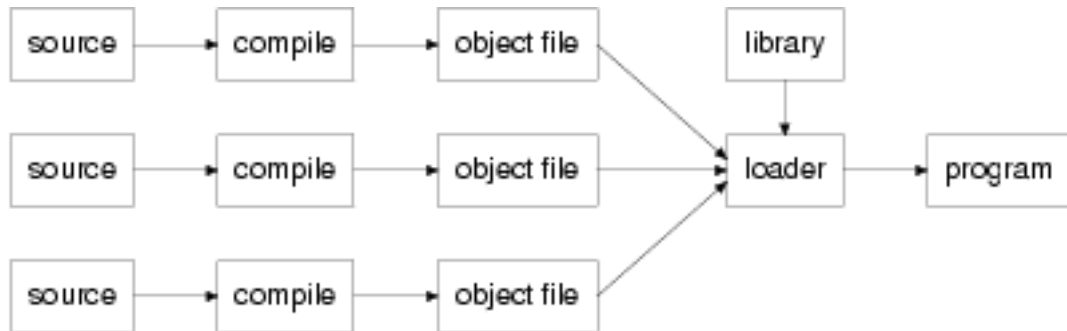
Figure 1.1: Diagram showing multiple files going from source, through compilation, to object files, and being combined with libraries by the loader to produce a program.
