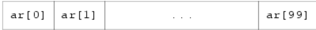
Figure 5.1: Diagram showing an array consisting of elements labelled 'ar[0]', 'ar[1]', etc., up to 'ar[99]'.
