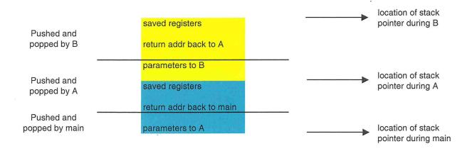
Yellow = what we need on the stack to support function B Blue = what we need on the stack to support function A
