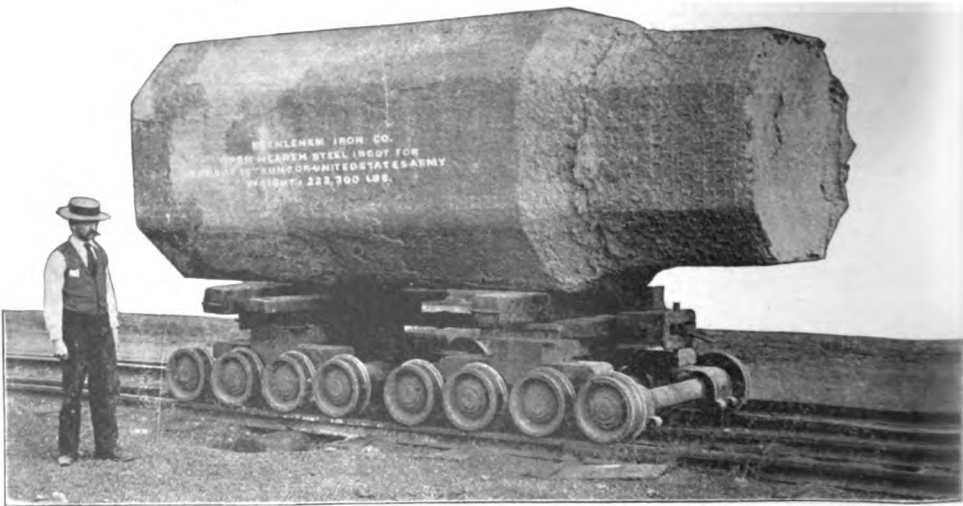
NICKEL STEEL INGOT CAST FOR THE TUBE OF 126-TON GUN. Manufactured for the United States Army by the Bethlehem Steel Co.
