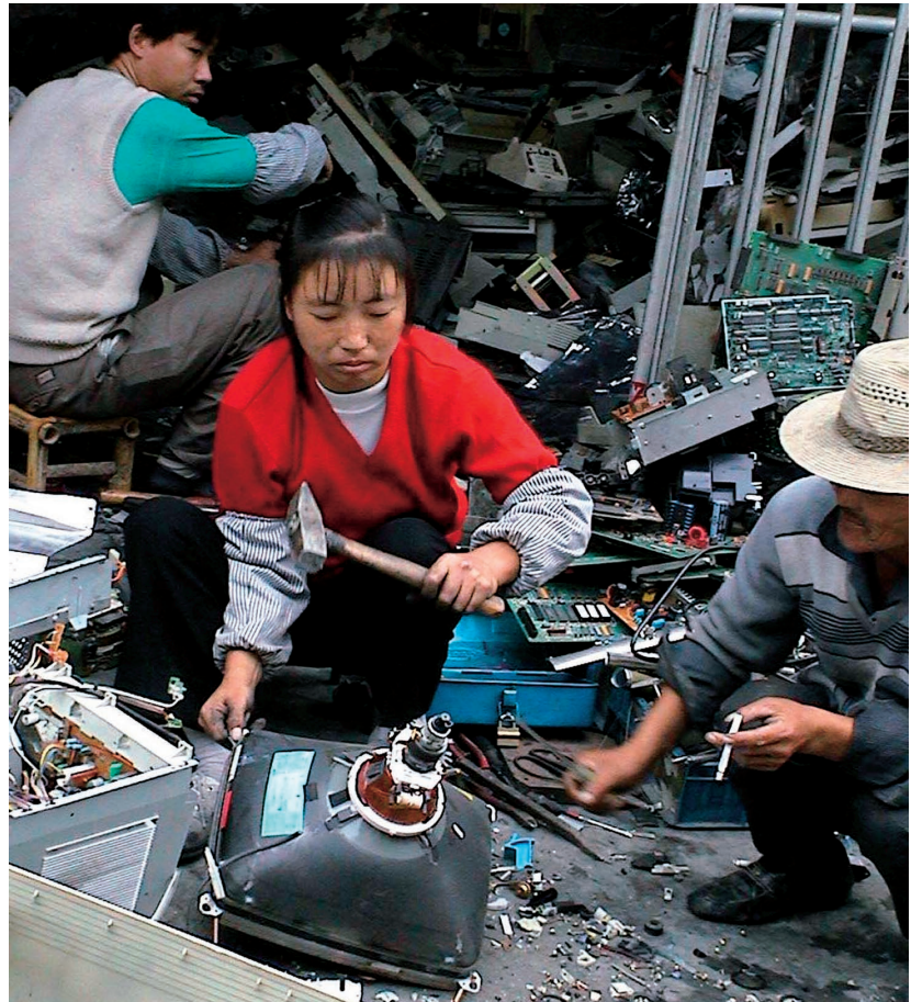
1 Woman in Guiyu, China smashing a cathode-ray tube from a computer monitor to remove the copper-laden yoke at the end of the funnel.
