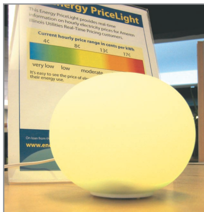
Figure 2. To help reduce summer electricity usage in Chicago, the Center for Neighborhood Technology created an ambient orb that displays households' real-time energy cost. Photo courtesy of CNT/CNT Energy.
