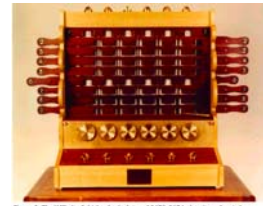
Figure 1. The William Schickard calculator of 1623–1624, showing a front view from an elevated position. The middle section is the adding machine with the result windows. The adding machine's base contains dials, which are used to enter the partial products that are taken from the multiplication and added. Notice the cybers on the right hand side, which is used to operate the calculator. The calculator's pedestal shows the memory unit's dial. (Photo courtesy of IBM Germany.)
