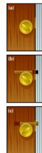
Figure 1.12 Deadbolt lock. (a) The external view. (b) Internal components, unlocked. (c) Internal components, locked. Thinking about how the deadbolt works allows us to see at a glance whether the door is locked or not.
