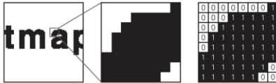
Figure 1.2. An enlargement of a monitor's display of the word bitmap and the corresponding bits for each pixel.
