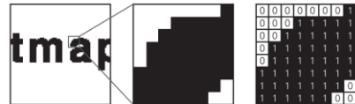
Figure 1.2. An enlargement of a monitor's display of the word bitmap and the corresponding bits for each pixel.
