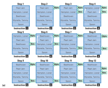
Figure 10.2. The steps of Alphabetize CDs algorithm. A snapshot of the CD rack is shown at the completion of each instruction. Notice how Beta sweeps through all of the slots following Alpha. After the first 11 steps, the alphabetically earliest CD, Beethoven, is in the Alpha slot.
