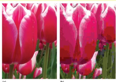
Figure 11.7. Detail from an image compressed using JPEG. (a) 14:1 compression (b) 140:1. Check images at www.aw.com/anyder
