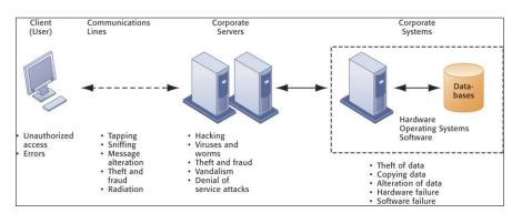
The architecture of a Web-based application typically includes a Web client, a server, and corporate information systems linked to databases. Each of these components presents security challenges and vulnerabilities. Floods, fires, power failures, and other electrical problems can cause disruptions at any point in the network.
