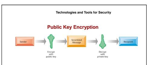
A public key encryption system can be viewed as a series of public and private keys that lock data when they are transmitted and unlock the data when they are received. The sender locates the recipient's public key in a directory and uses it to encrypt a message. The message is sent in encrypted form over the Internet or a private network. When the encrypted message arrives, the recipient uses his or her private key to decrypt the data and read the message.
