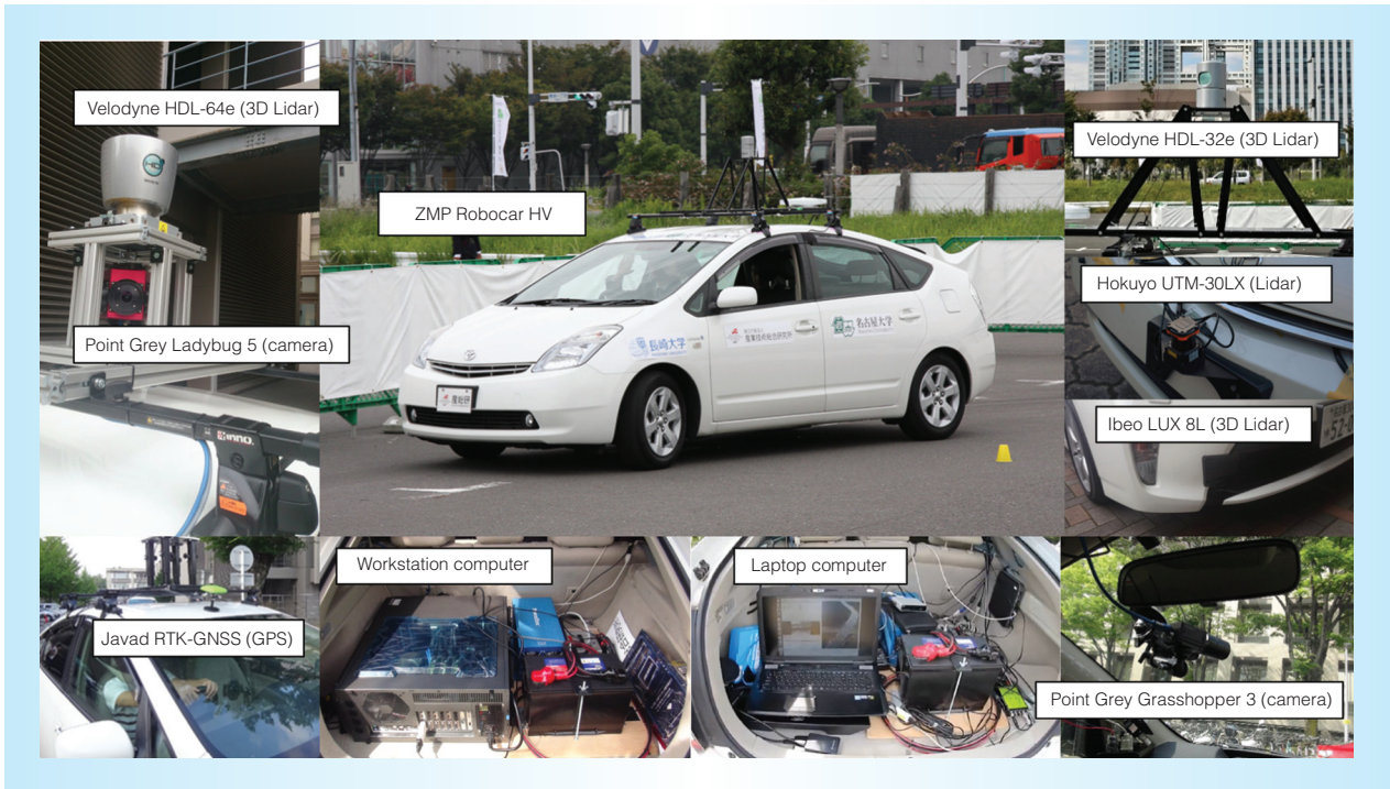
Figure 1. ZMP Robocar “HV” and examples of sensors and plug-in computers. Omni view cameras, Lidar sensors and GNSS receivers are equipped outside of the vehicle, while single-view cameras and computers are set inside.
